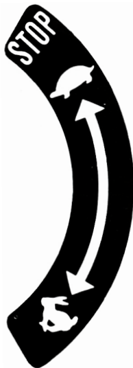
Hand Throttle Control Lever PART NO. – SBA-390430100. LOCATION – Hand throttle lever, right side of instrument panel.
